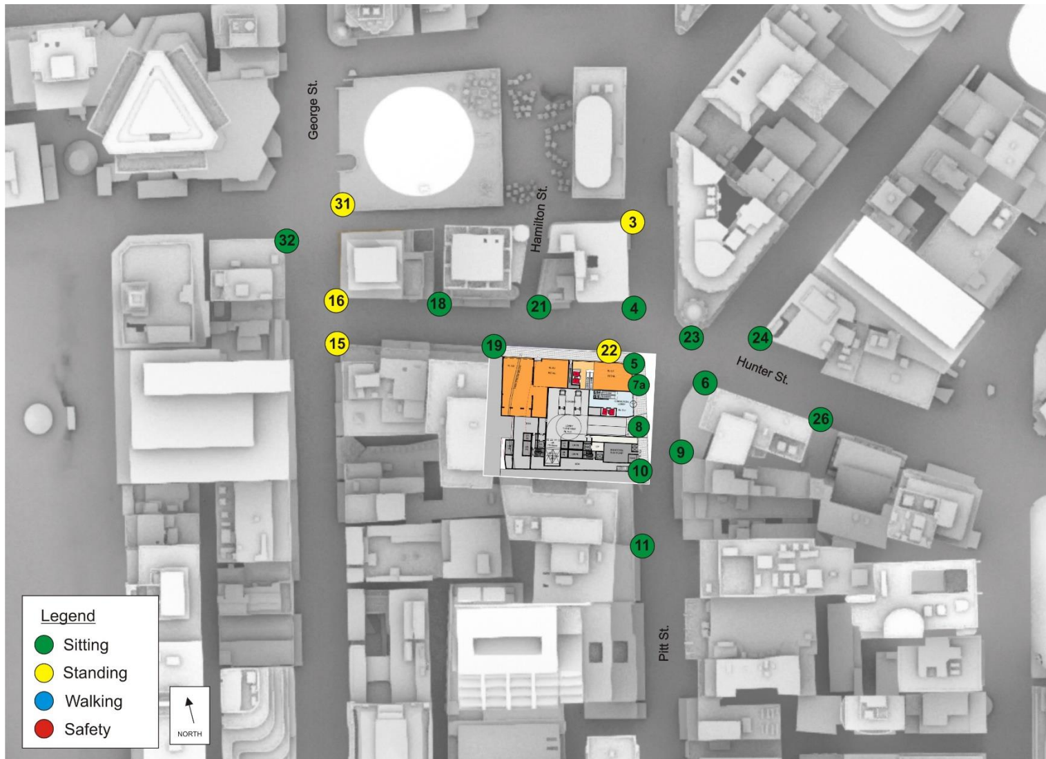
Figure 7 – Summary of ground level wind conditions for the Base Case Configuration for 360° of wind direction.
